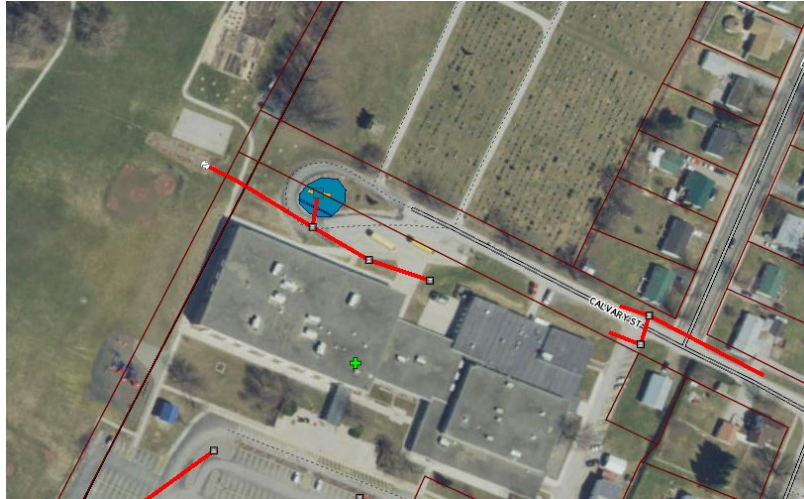
Figure 7. Outfall 54 can be seen at the end of the stormline. The blue polygon indicates an existing rain garden on the map.
